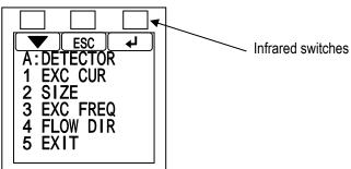
(2) Switch position: BOTTOM (Standard) The infrared switches are located at the bottom with the front facing you.
